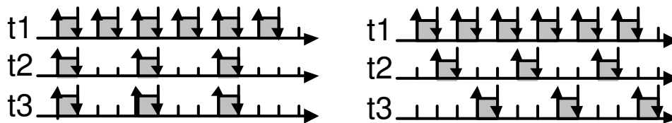
Figure 11: left: Unfeasible schedule of tasks with periodic access. right: Same task set becomes feasible due to adding appropriate phase to some tasks.
